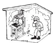
any enclosed or narrow area where free flow of the air is restricted. If the air flow is restricted it will cause serious damage to the saw's engine and may cause injury to people. Remember the saw's engine gives off **DEADLY** carbon monoxide gas.
